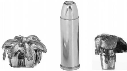
When bullets hit their targets, the soft lead deforms. The high-performance, expensive bullet on the left has “opened up” almost perfectly, whereas the one on the right has not.
