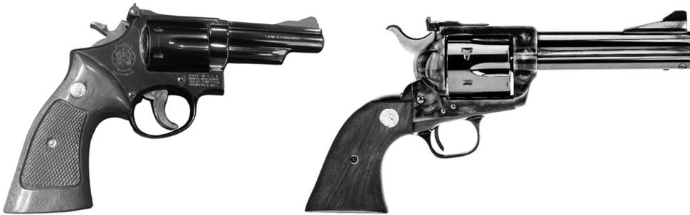
The two main types of revolvers. Left: Double-action revolver (Smith & Wesson Model 19). Right: Single-action revolver (Colt Single Action Army, colloquially known as the “Peacemaker”). An observer will note that on any single action, the trigger will be very close to the back of the trigger guard because the trigger pull need only release the already cocked hammer. On a double action, the trigger must also pull the hammer back.
