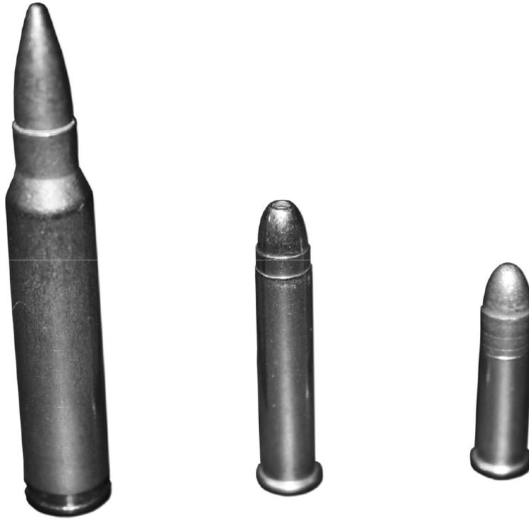
Different types of ammunition. From left to right, .223 Remington, .22 WMR, and .22 LR. Note that the bullet (the top part) for the .223 Remington is only  $\frac{3}{1000}$  of an inch wider than the .22 caliber bullets. But the .223 Remington's case is much wider and larger, allowing more room for gunpowder, making it far more powerful than the other two.
