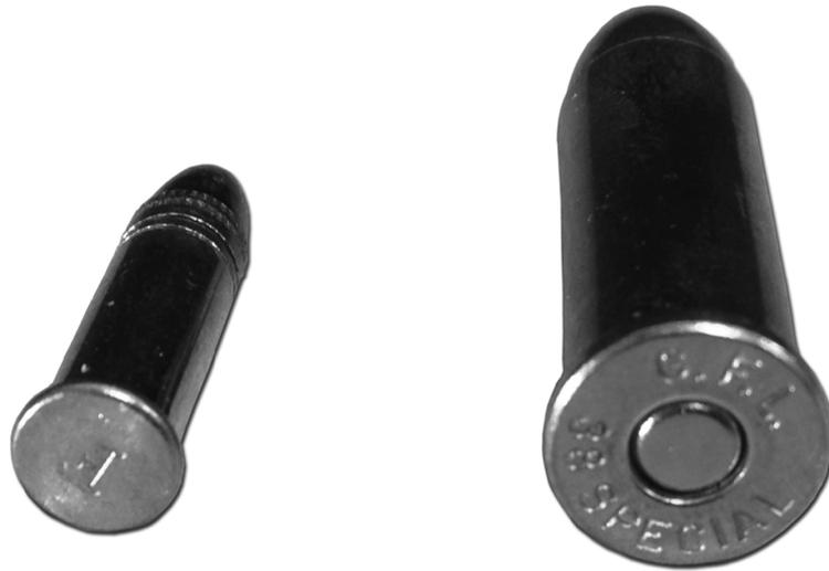
Rimfire vs. centerfire cartridges. At left is a .22 Long Rifle round, a rimfire cartridge. At right is a .38 Special round, a centerfire cartridge. Note the telltale, circular primer cup that sits at the bottom of the centerfire cartridge's case head. The rimfire cartridge lacks this. Instead, it has a layer of priming compound (not visible) applied to the inside of the brass rim of the cartridge.
