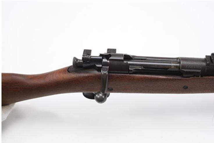
Close-up of the action of the 1903 Springfield. The bolt is operated by the handle that has a large ball at the end. To eject an empty shell casing, the user moves the handle up and then back. To load a fresh round, the user then moves the handle forward and down. The box magazine, which is not pictured, attaches at the bottom of the rifle, in front of the trigger guard.
